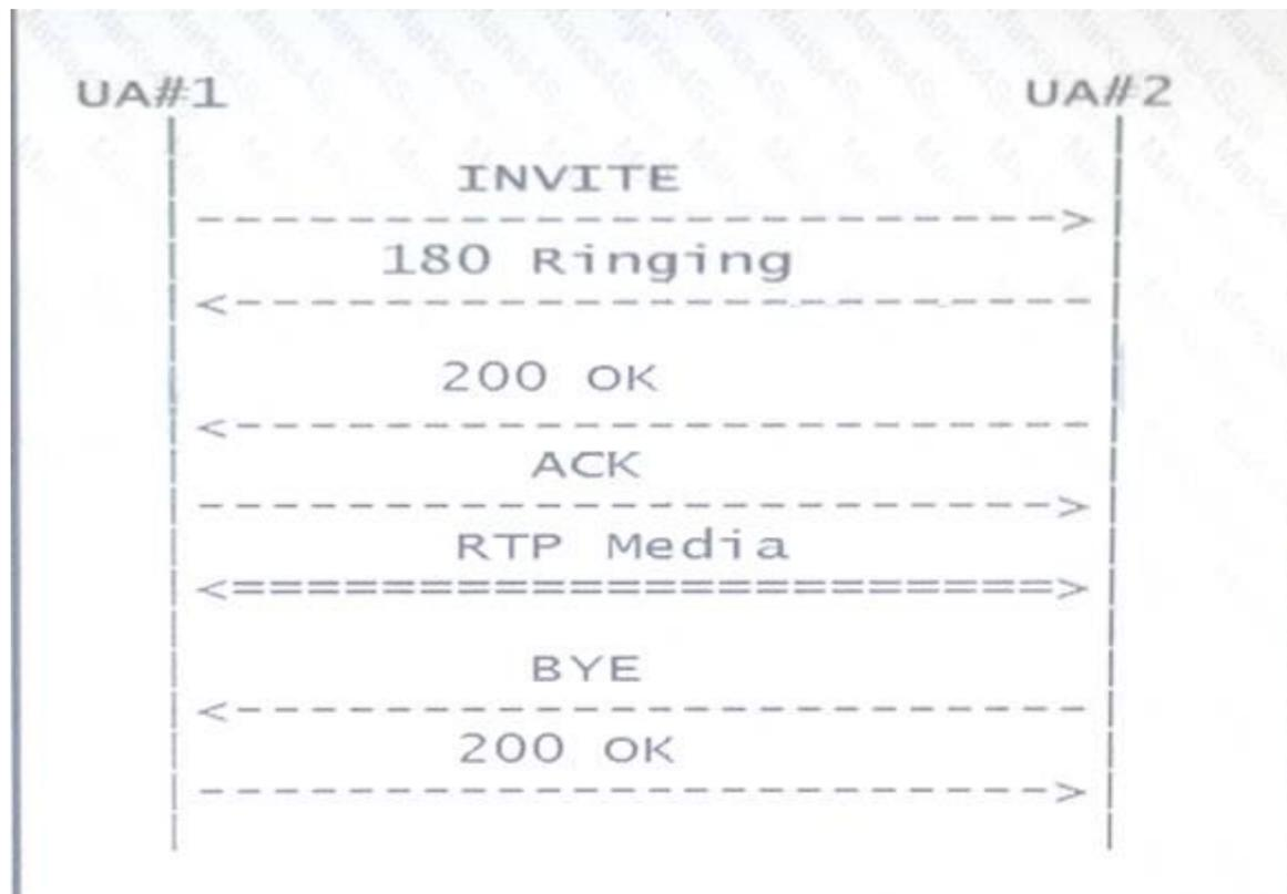
How many SIP signalling transaction(s) took place in this SIP message exchange between two SIP user agents?
