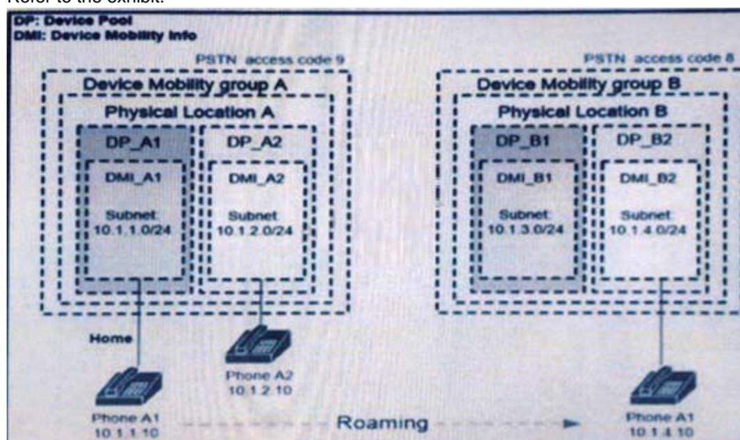
A collaboration engineer is configuring device mobility. Which three occur to phone A1 when it moves to physical location B? (Choose three)
