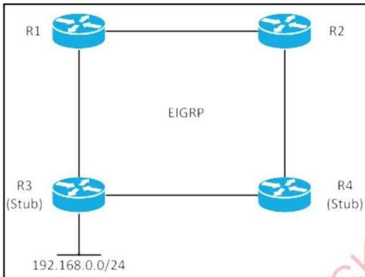
All routers are running EIGRP and the network has converged. R3 and R4 are configured as EIGRP Stub. if the link between R1 and R3 goes down, which statement is true?
