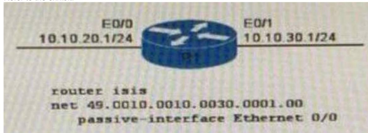
If router R1 is configured to run IS-IS with given configuration and all interfaces are up/up, what action must you take so that the Ethernet 0/0 network can be advertised to potential IS-IS neighbors on the E0/1 interface?
