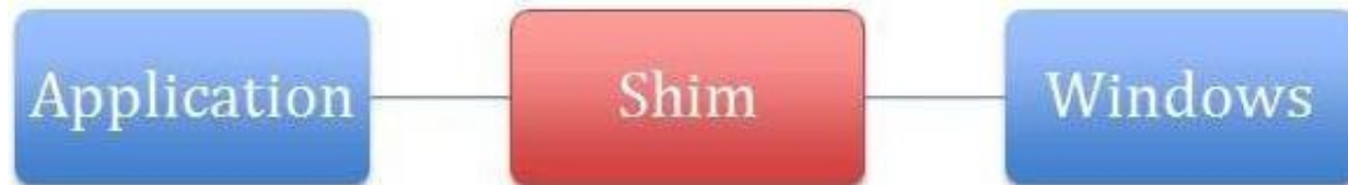
Figure 2 After the shim is applied, the application interacts with Windows indirectly; the shim code is injected and can modify the request to Windows, the response from Windows, or both.
