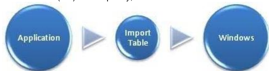
Figure 1 Application calling into Windows through the IAT Specifically, you can modify the address of the Windows function resolved in the import table, and then replace it with a pointer to a function in the alternate shim code, as shown in Figure 2
