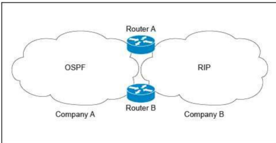
Company A is running a single-area OSPF, and Company B is running RIP as the IGP with no overlapping IP address spaces. Company A has just acquired Company B and both networks must be merged. Which three design components are recommended to guarantee connectivity and redundancy between the two networks? (Choose three.)
