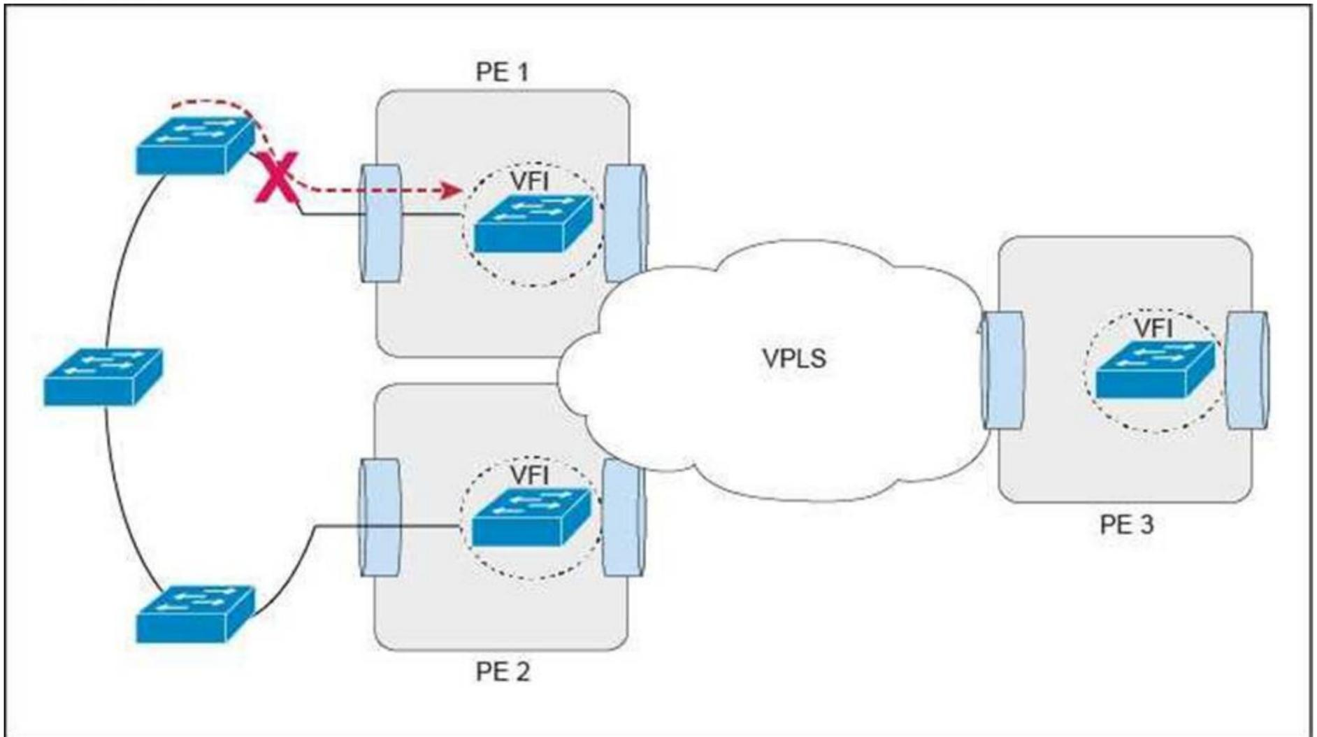
This Layer 2 ring has 10 VLANs with 1000 MAC addresses in each VLAN. Which protocol or mechanism provides the shortest traffic outage if the link marked with "X" fails?
