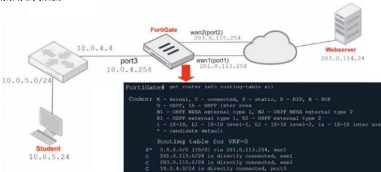
Which contains a network diagram and routing table output. The Student is unable to access Webserver.
