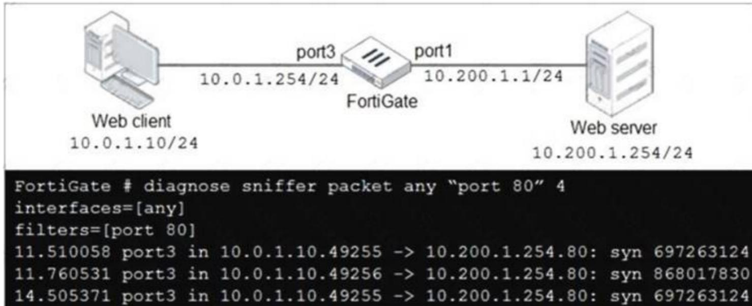
In the network shown in the exhibit, the web client cannot connect to the HTTP web server. The administrator runs the FortiGate built-in sniffer and gets the output as shown in the exhibit.
