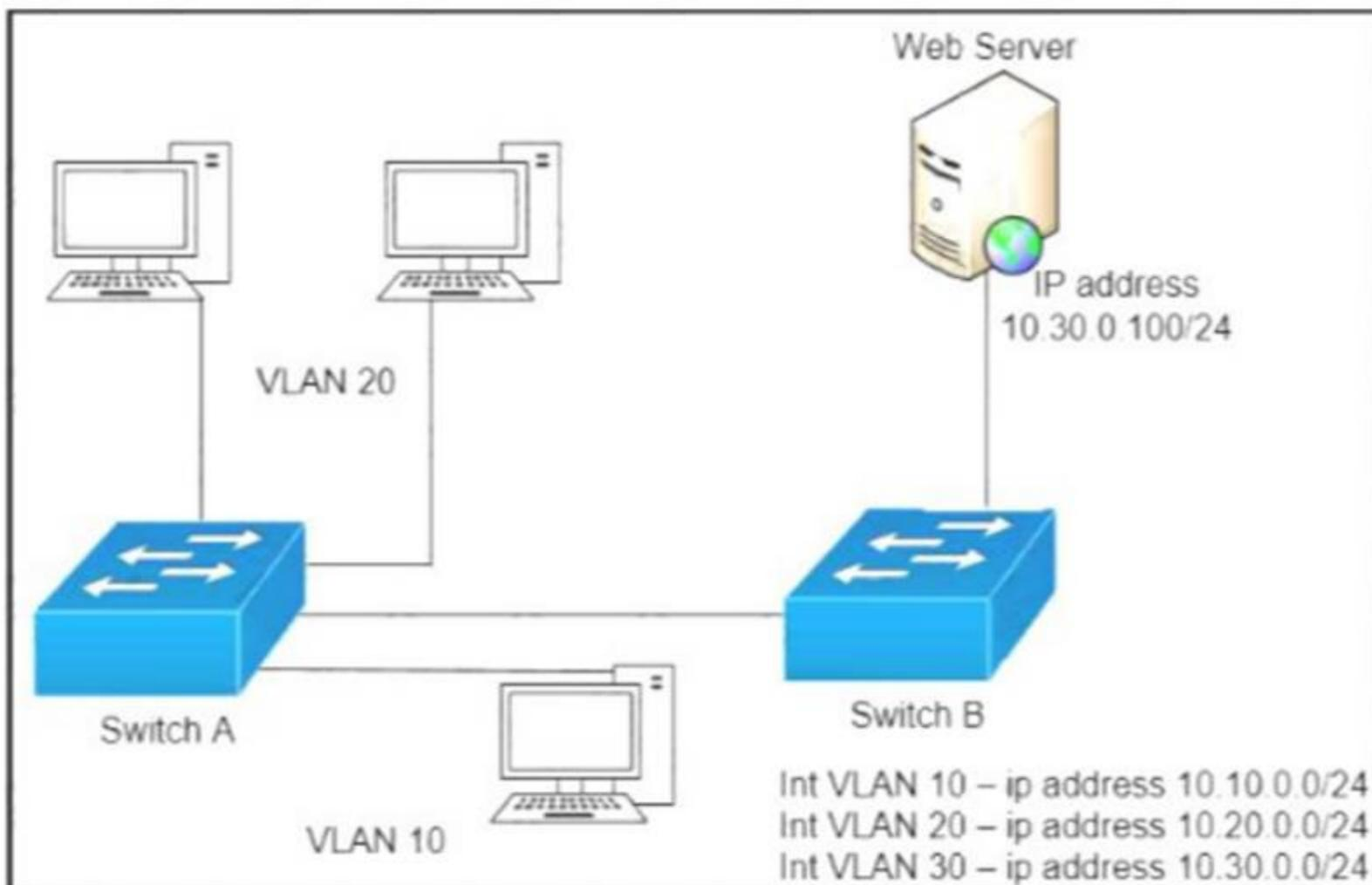
A network engineer must block access for all computers on VLAN 20 to the web server via HTTP. All other computers must be able to access the web server. Which configuration when applied to switch A accomplishes this task?
