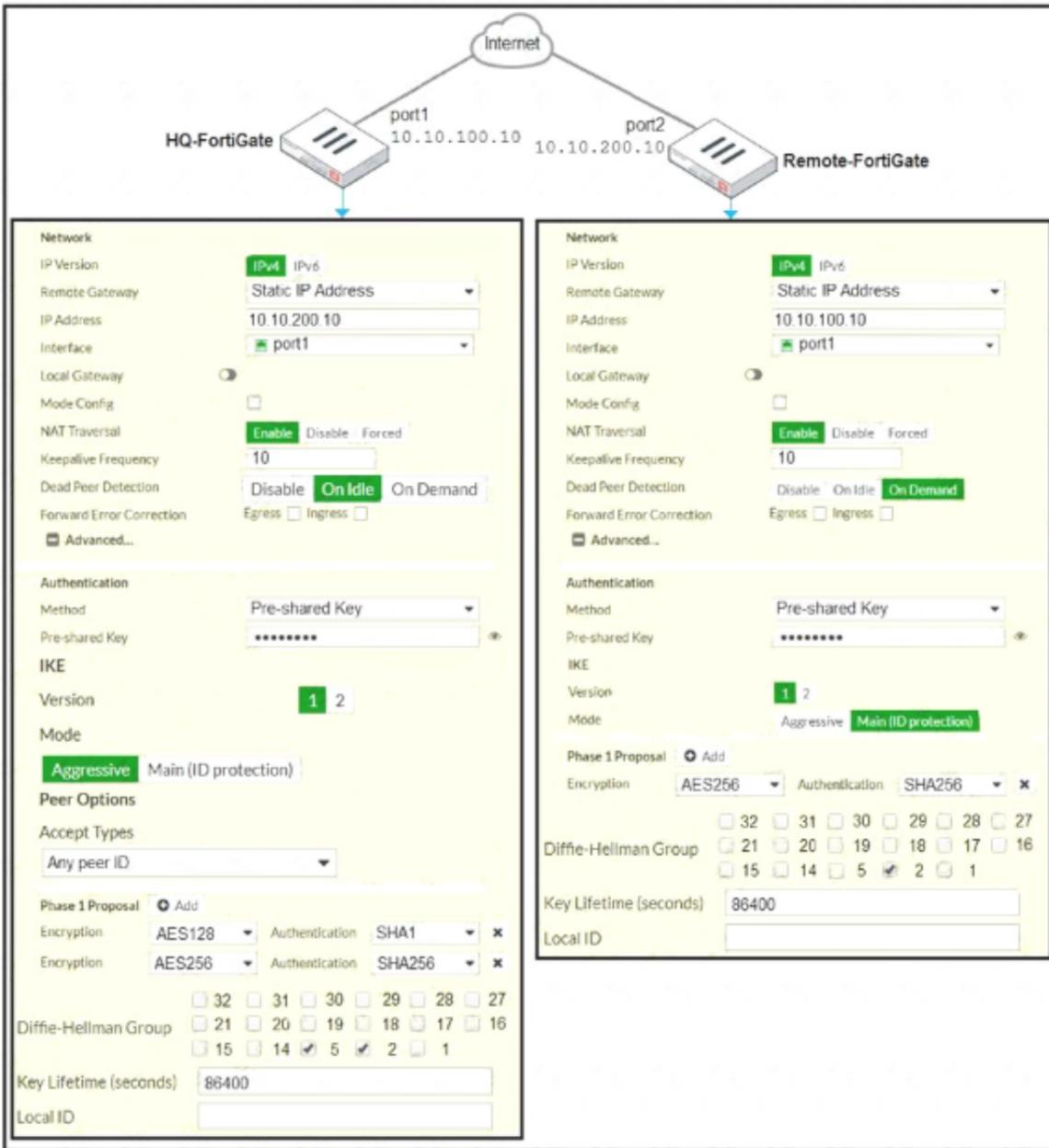
A network administrator is troubleshooting an IPsec tunnel between two FortiGate devices. The administrator has determined that phase 1 fails to come up. The administrator has also re-entered the pre-shared key on both FortiGate devices to make sure they match. Based on the phase 1 configuration and the diagram shown in the exhibit, which two configuration changes will bring phase 1 up? (Choose two.)
