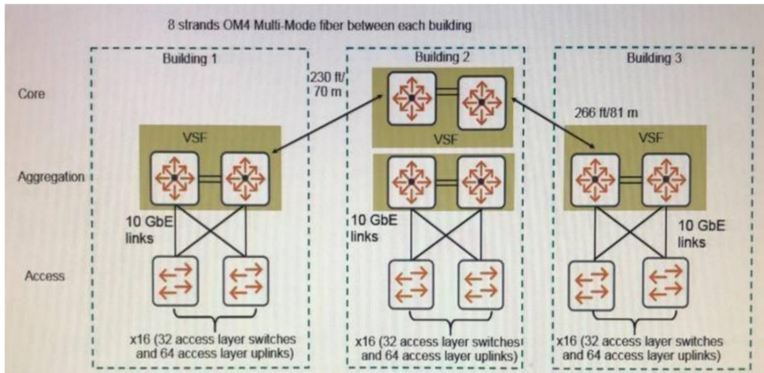
An architect selects 5406R switches for the aggregation layer. What is an appropriate amount of bandwidth for the link aggregation between each aggregation layer VSF fabric and the campus core?
