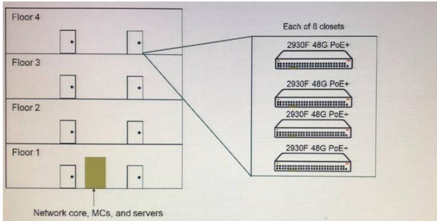
An architect needs to plan a network solution for a new office building with four floors. Each floor has two wiring closets with the equipment shown in the exhibit. The switches will connect to employee desktops, a few campus APs controlled by MCs, and printers. The switches do not implement tunneled node. What is a best practice design for the VLANs and subnets for the wired devices?
