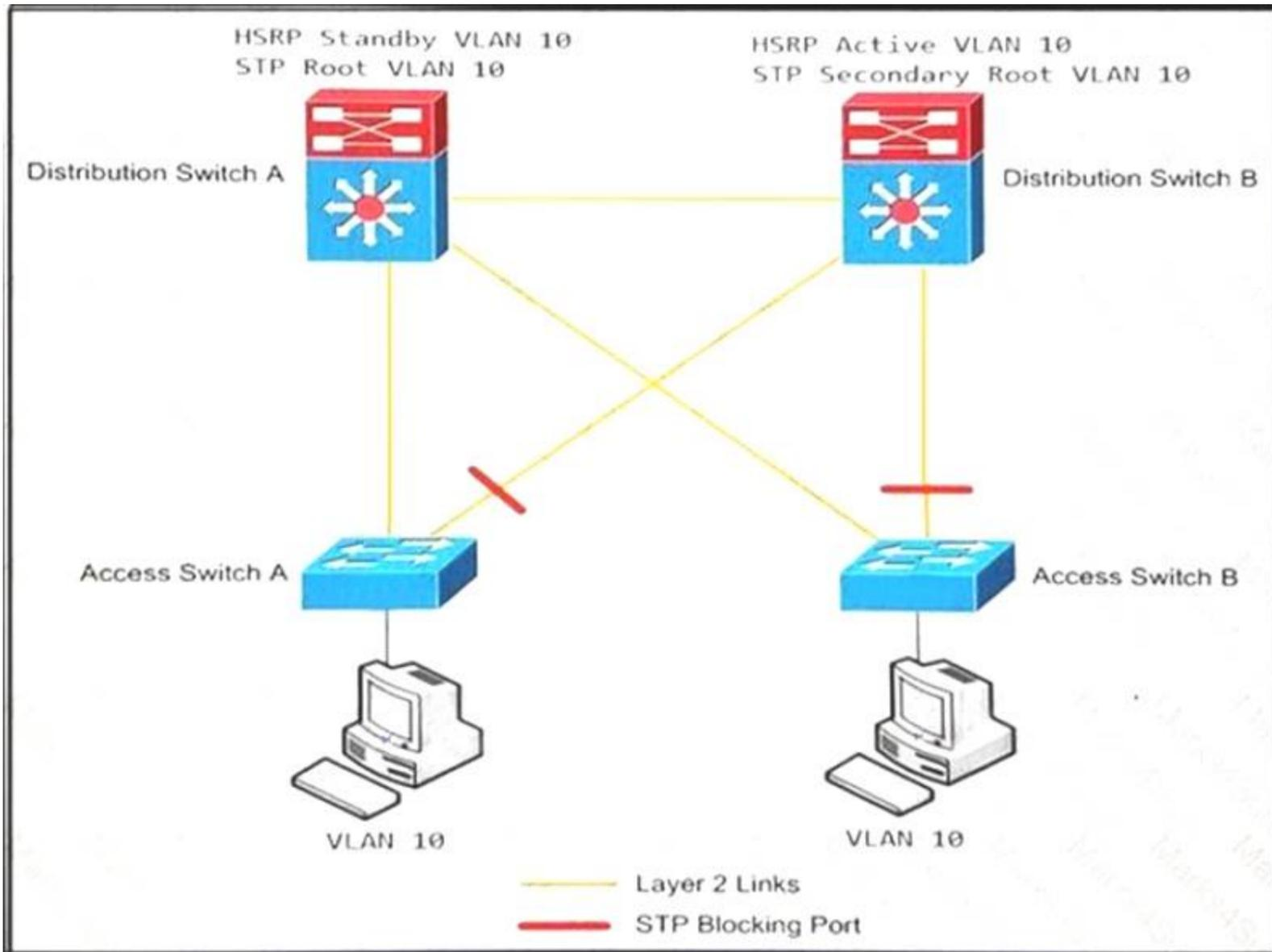
An engineer must optimize the traffic flow of the network. Which change provides a more efficient design between the access and the distribution layer?
