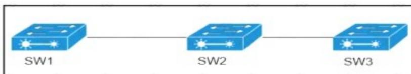
VLANs 50 and 60 exist on the trunk links between all switches. All access ports on SW3 are configured for VLAN 50 and SW1 is the VTP server. Which command ensures that SW3 receives frames only from VLAN 50?
