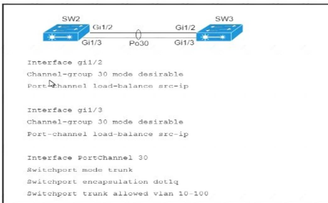
A port channel is configured between SW2 and SW3. SW2 is not running a Cisco operating system. When all physical connections are made, the port channel does not establish. Based on the configuration excerpt of SW3, what is the cause of the problem?
