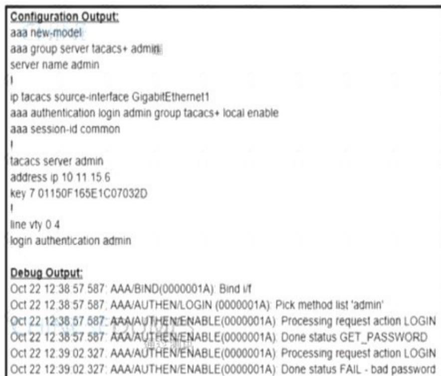
An administrator configured a Cisco router for TACACS authentication, but the router is using the local enable password instead Which action resolves the issue?
