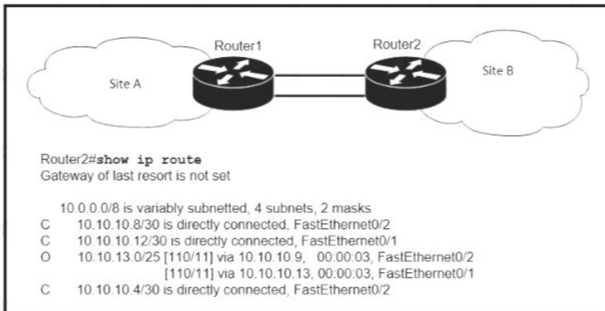
If OSPF is running on this network, how does Router 2 handle traffic from Site B to 10.10.13/25 at Site A?
