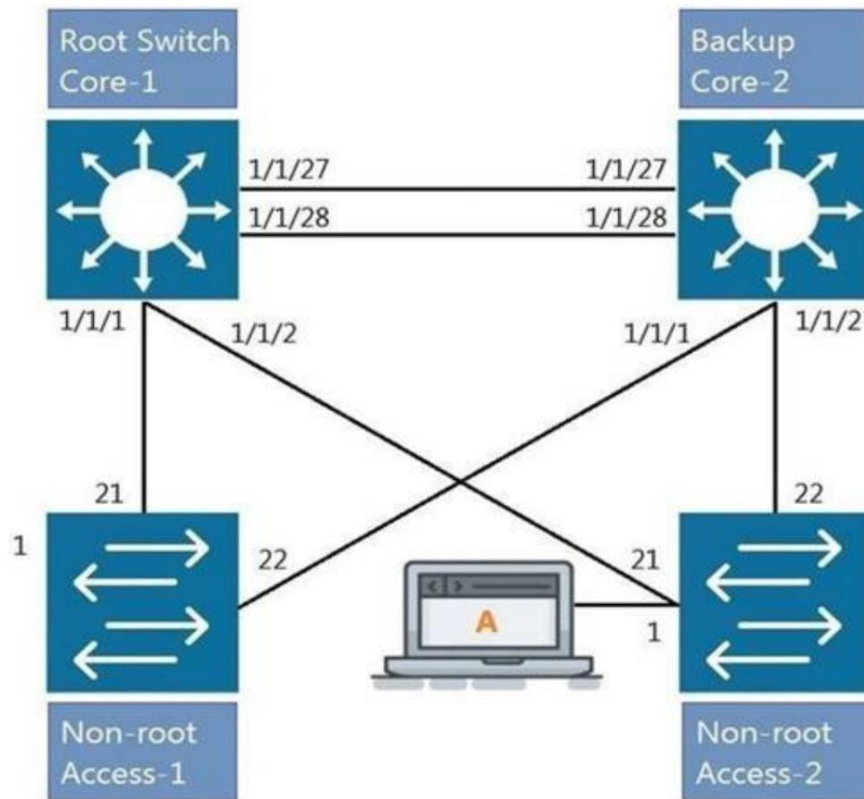
All four switches in the diagram have been configured with the region name "Aruba1". What two other MSTP configurations must match for switches within the same MST region? (Choose two.)
