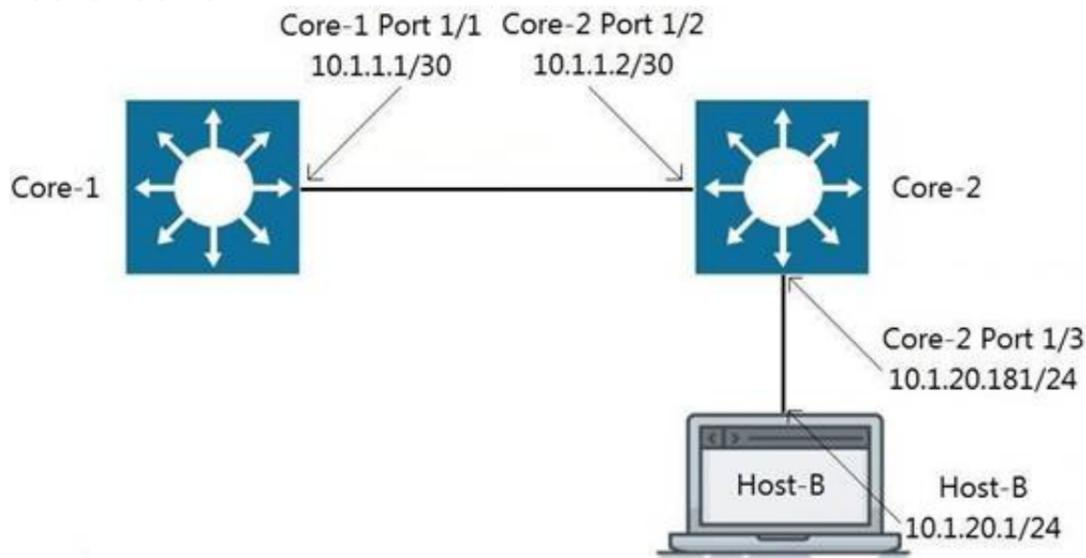
Traffic is failing between Core-1 and Host-B. IP addressing has correctly been applied, and all interfaces are attached to the vrf GREEN. Which configuration will correct the issue?
