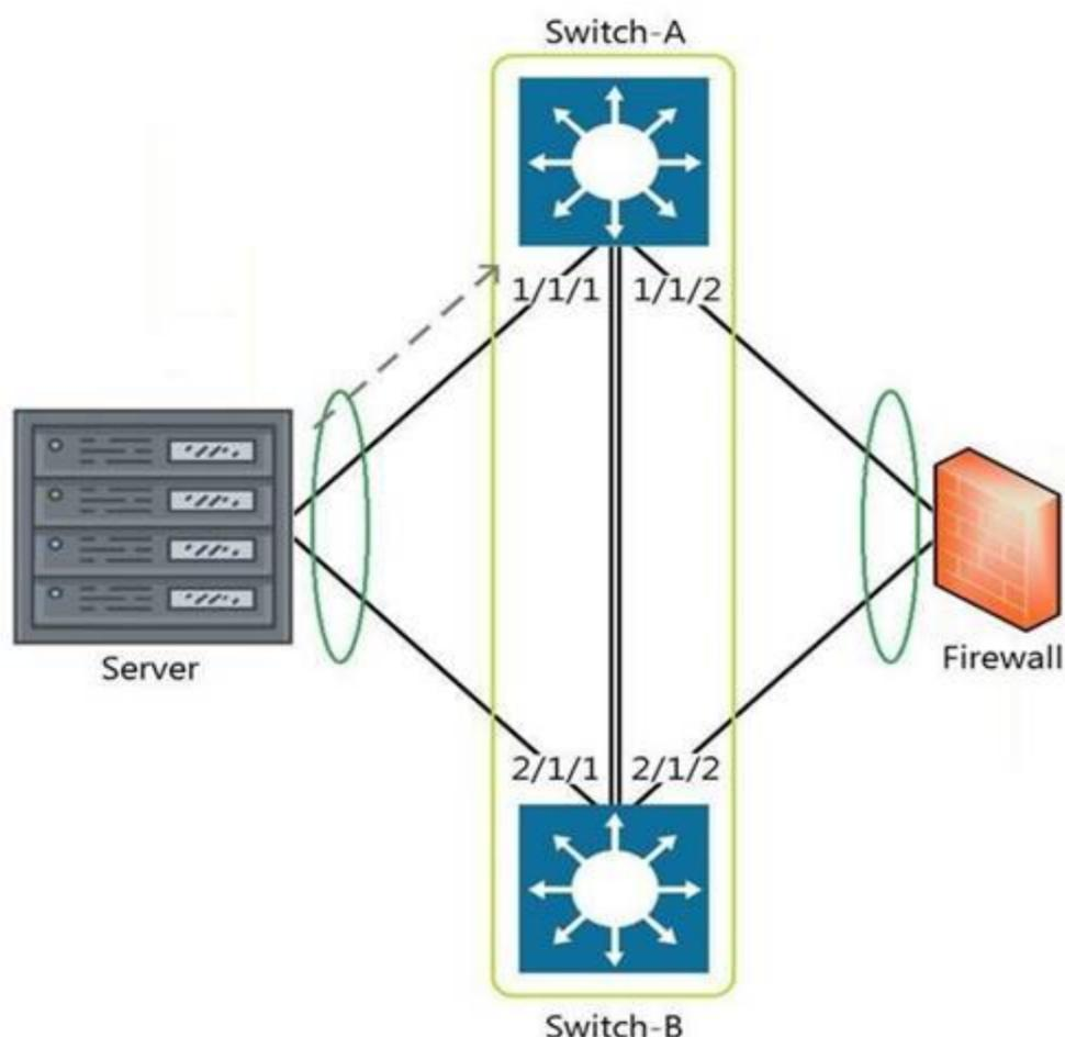
The above scenario shows a packet from the Server destined for the Firewall. Switch-A and Switch-B are bundled as VSF stack. The LAG between the VSF stack and the firewall indicates a hash function to forward the packet on port 2/1/2.
