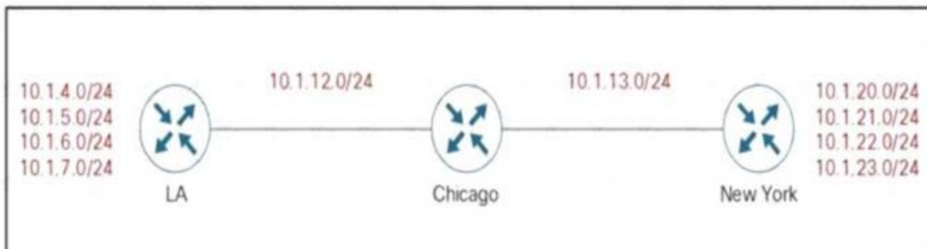
Company XYZ BGP topology is as shown in the diagram. The interface on the LA router connected toward the 10.1.5.0/24 network is faulty and is going up and down, which affects the entire routing domain. Which routing technique can be used in the routing policy design so that the rest of the network is not affected by the flapping issue?
