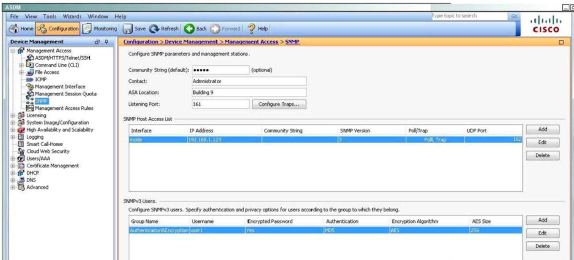
SNMP users have a specified username, a group to which the user belongs, authentication password, encryption password, and authentication and encryption algorithms to use. The authentication algorithm options are MD5 and SH
