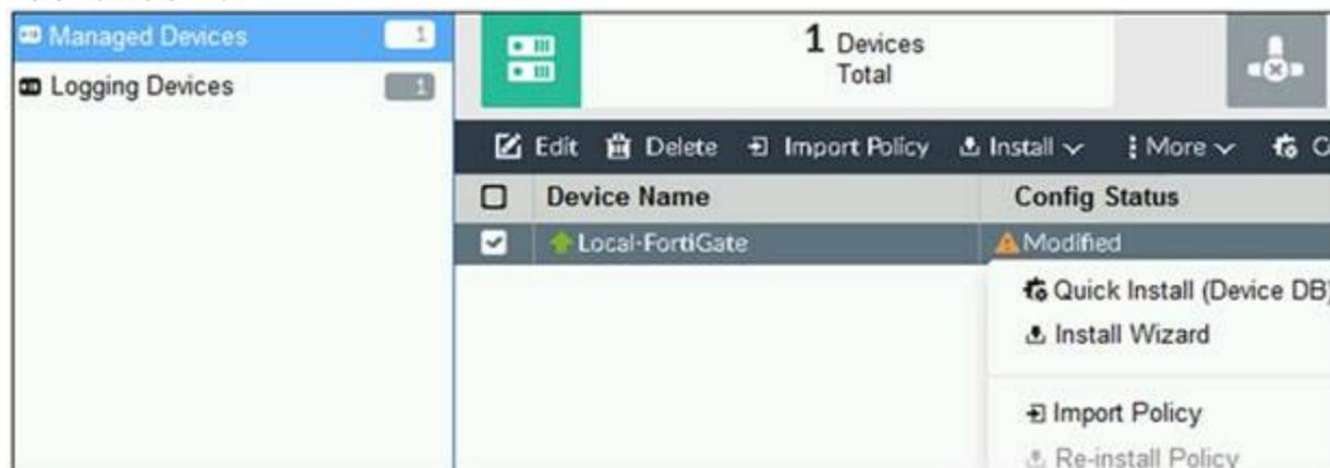
You are using the Quick Install option to install configuration changes on the managed FortiGate.
