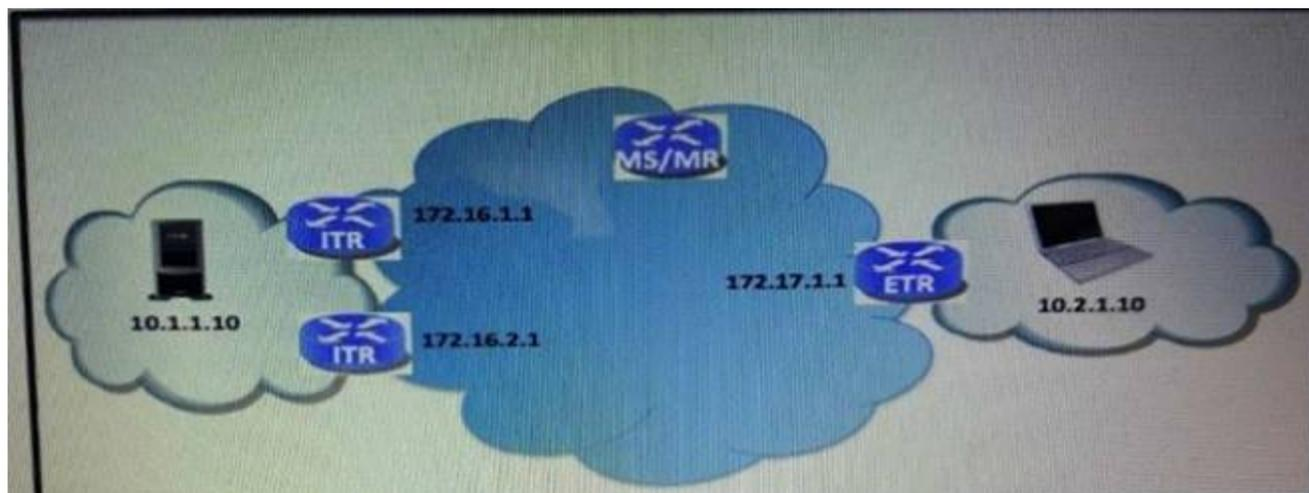
Refer to the exhibit. The ITR map cache is empty. The ITR receives packet destined for 10.2.1.10 and it sends query to the MR. Which action does the MR/MS take after receive the query for 10.2.1.10?
