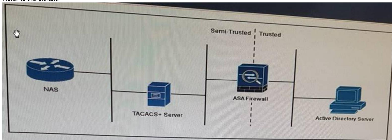
A user authenticates to the NAS, which communicates to the TACACS+ server for authentication. The TACACS+ server then accesses the Active Directory Server through the firewall to validate the user credentials. Which protocol-port pair must be allowed access through the ASA Firewall?
