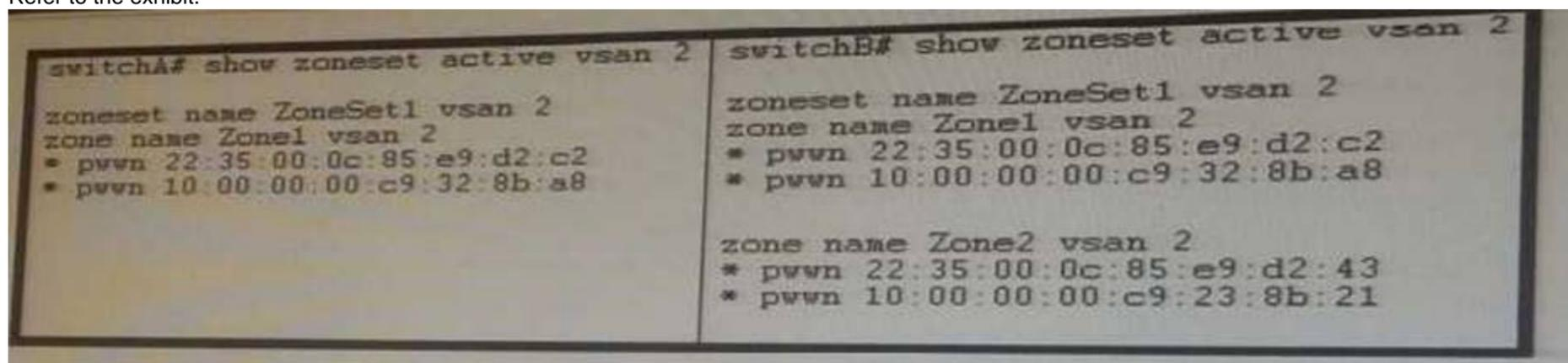
Refer to the exhibit. Switch A and switch B have these zone sets currently active and are connected by an ISL that is configured to transport VSAN 2 Enhanced zoning is configured for VSAN 2 and merge-control is set to restrict. Which statement about this configuration is true?
