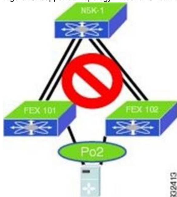
If you need to connect a multi-homing server to a pair of FEXs when there is only one Cisco Nexus 5000 Series device, you have the option to run active or standby NIC teaming from the server. Reference: [http://www.cisco.com/en/US/docs/switches/datacenter/nexus5000/sw/mkt\\_ops\\_guides/513\\_n1\\_1/n5k\\_enhanced\\_vpc.html](http://www.cisco.com/en/US/docs/switches/datacenter/nexus5000/sw/mkt_ops_guides/513_n1_1/n5k_enhanced_vpc.html)
