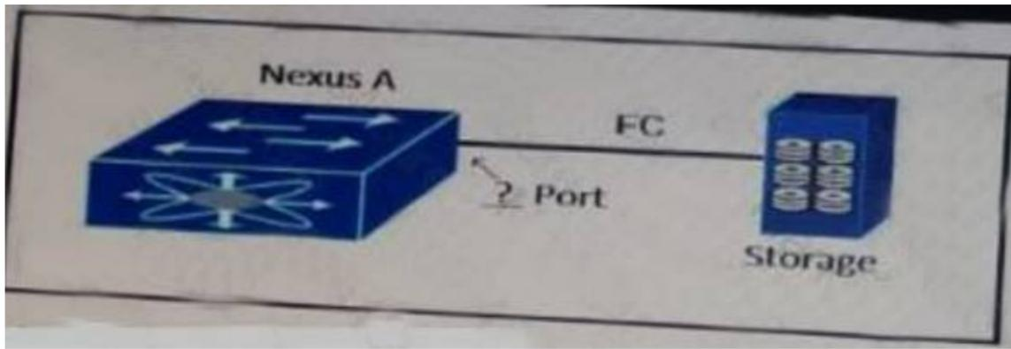
You must attach a storage peripheral to a Cisco Nexus 5000 Series Switch. Which type of port do you use?
