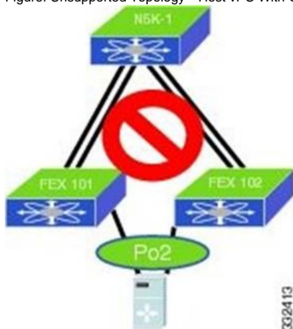
If you need to connect a multi-homing server to a pair of FEXs when there is only one Cisco Nexus 5500 Series device, you have the option to run active or standby NIC teaming from the server. Reference: [http://www.cisco.com/en/US/docs/switches/datacenter/nexus5000/sw/mkt\\_ops\\_guides/513\\_n1\\_1/n5k\\_enhanced\\_vpc.html](http://www.cisco.com/en/US/docs/switches/datacenter/nexus5000/sw/mkt_ops_guides/513_n1_1/n5k_enhanced_vpc.html)
