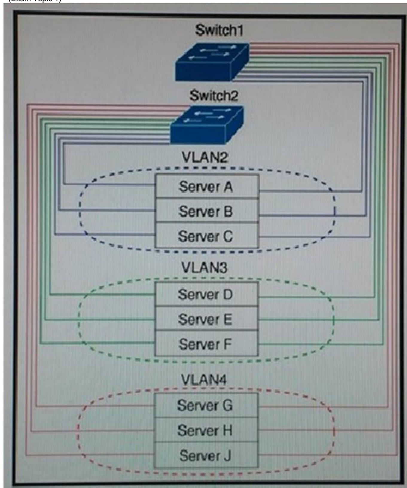
Refer to the exhibit. Two Layer 2 Cisco Nexus switches are connected to application servers in a data center. Server A cannot communicate with servers that are in VLANs 3 and 4, but it can communicate with server B and C. What is the cause of the problem?
